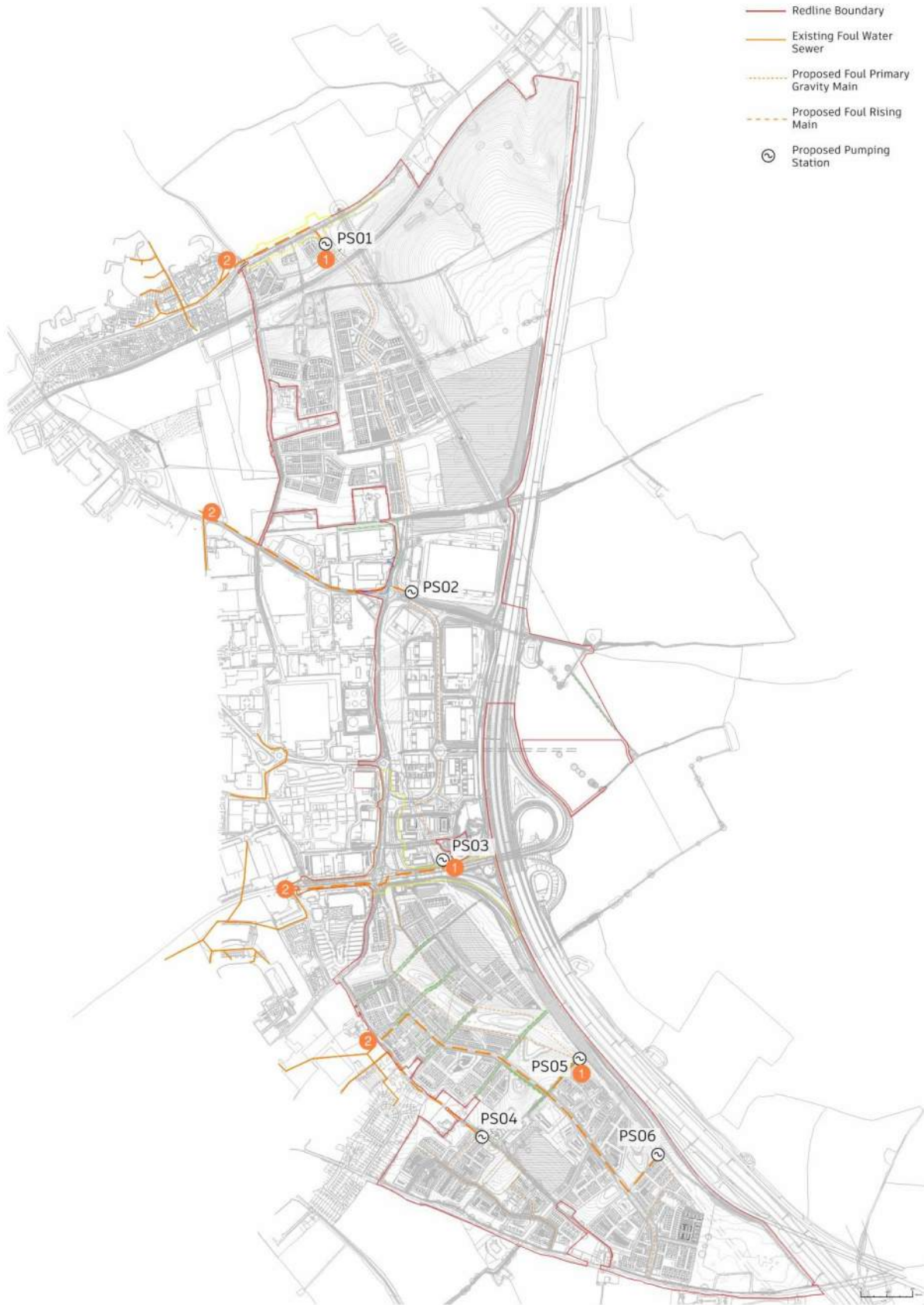
Figure 18: Propose foul water sewer network where (1) identifies pumping locations and (2) identifies possible points of connection
