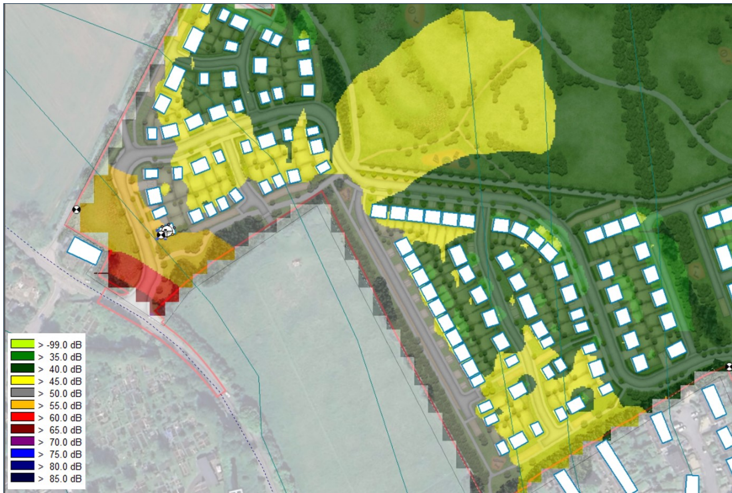
Figure 11.4 Areas Requiring Acoustic Fencing
