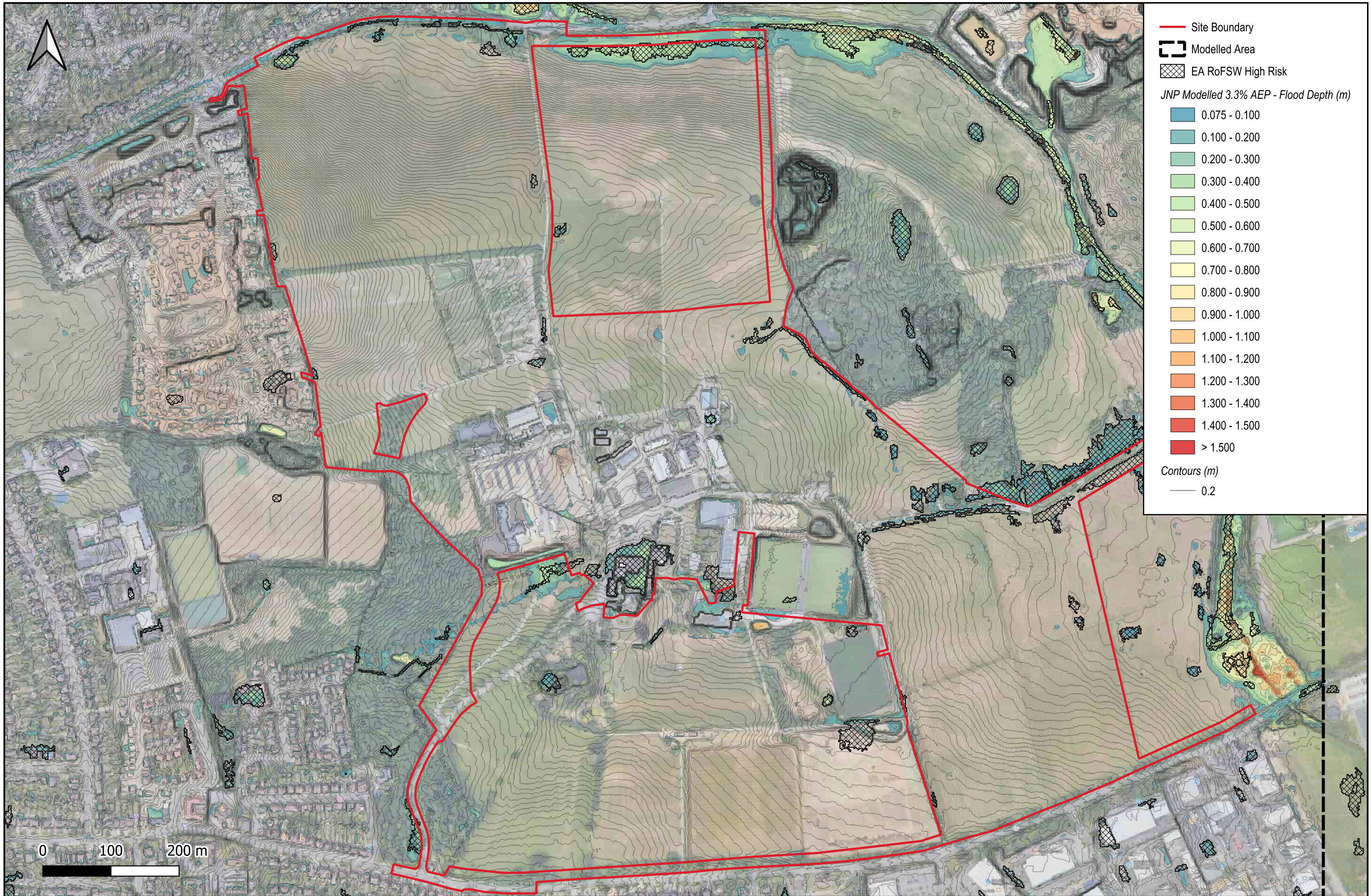
Map 06 - Sandpit Lane - Existing Baseline 1hr 3.3% AEP JNP modelled against EA - Max Flood Depth
