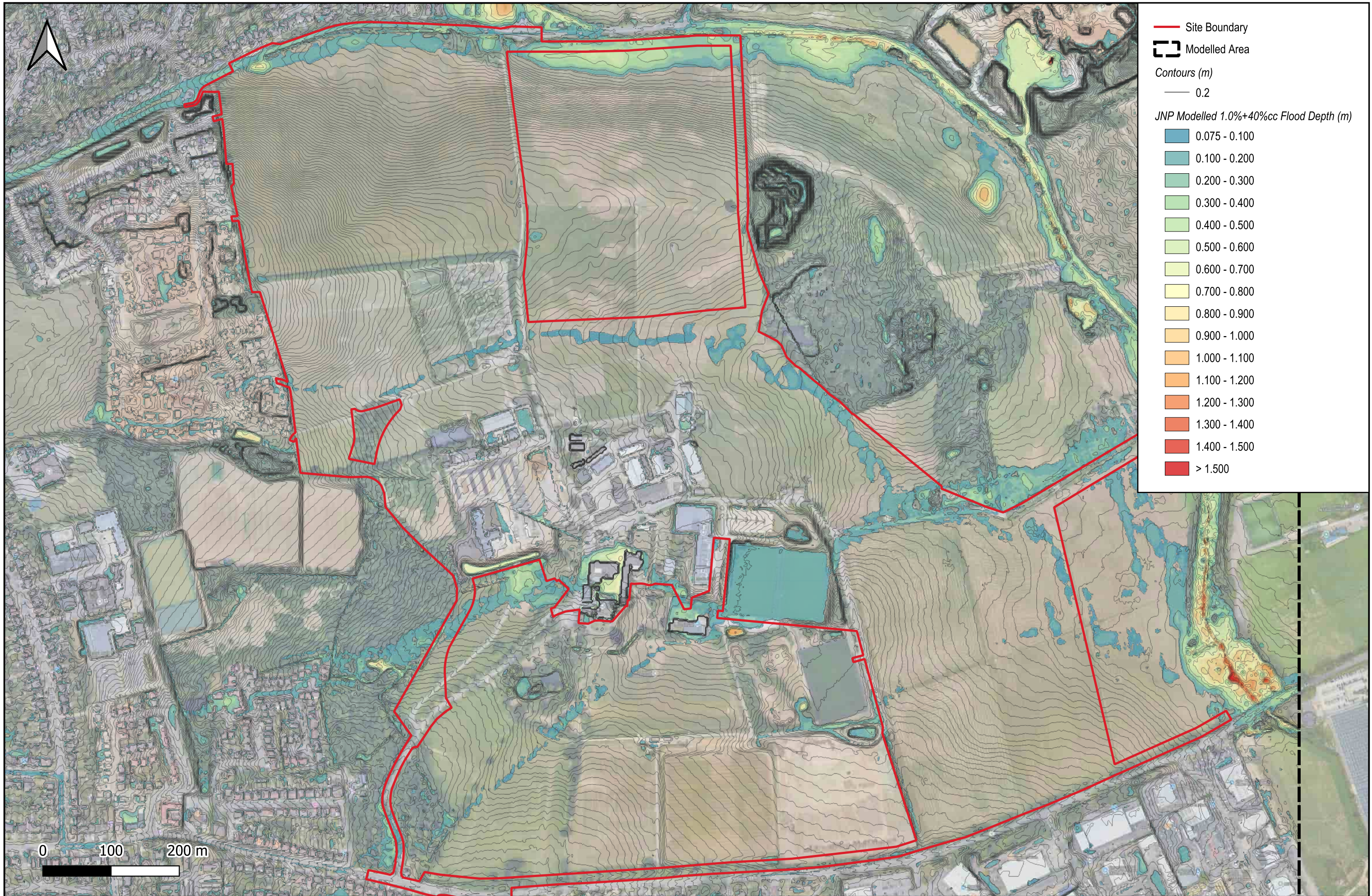
Map 07 - Sandpit Lane - Existing Baseline 1hr 1.0% AEP + 40% cc - Max Flood Depth
