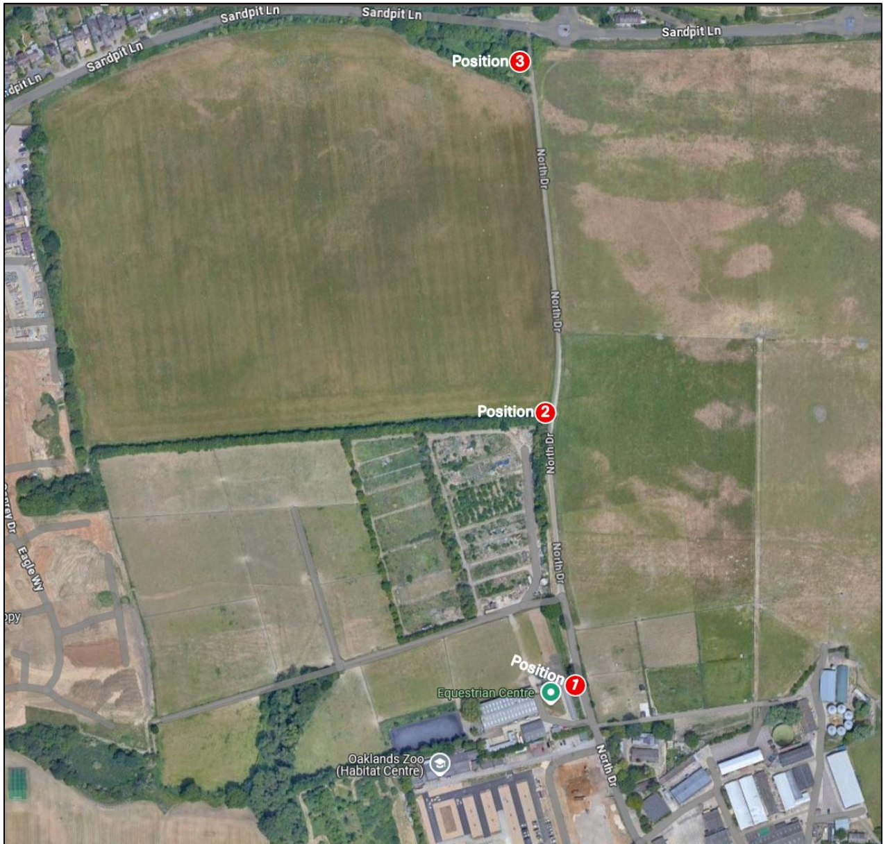
Figure 3 - Noise monitoring locations on site
